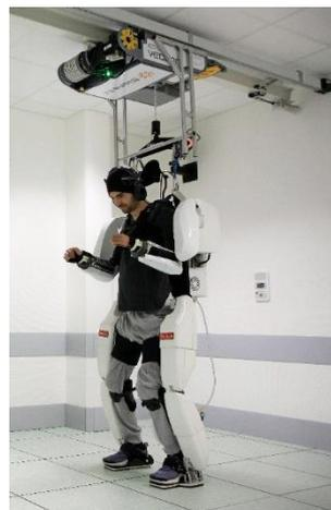
The four-limb exoskeleton controlled by the patient during the BCI project at Clinatec ©Clinatec
